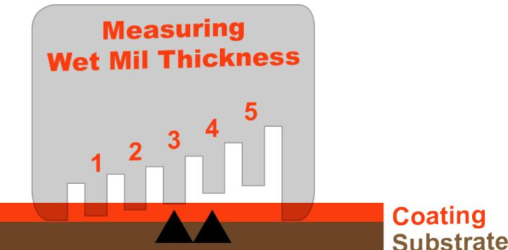
A wet film gauge is required to be 100% precise. It is recommended that you check the wet film thickness every three feet to ensure 100% accuracy.
