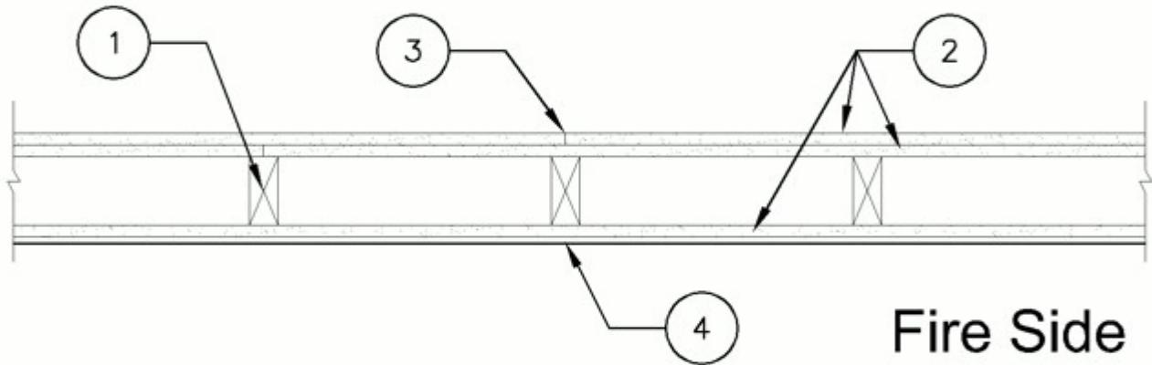
1. **Wood Studs** — Nom 2 by 4 in. spaced 16 in. OC max, with blocking installed at mid-height.
